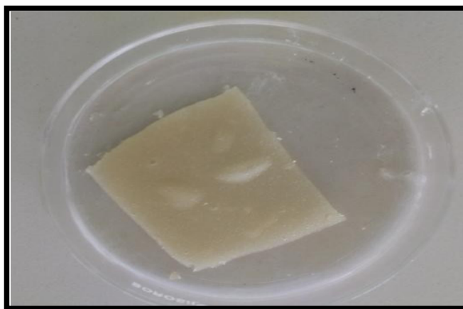
Figure-3. Surface view of prepared transdermal patch recovered after 24hrs of solvent evaporation
